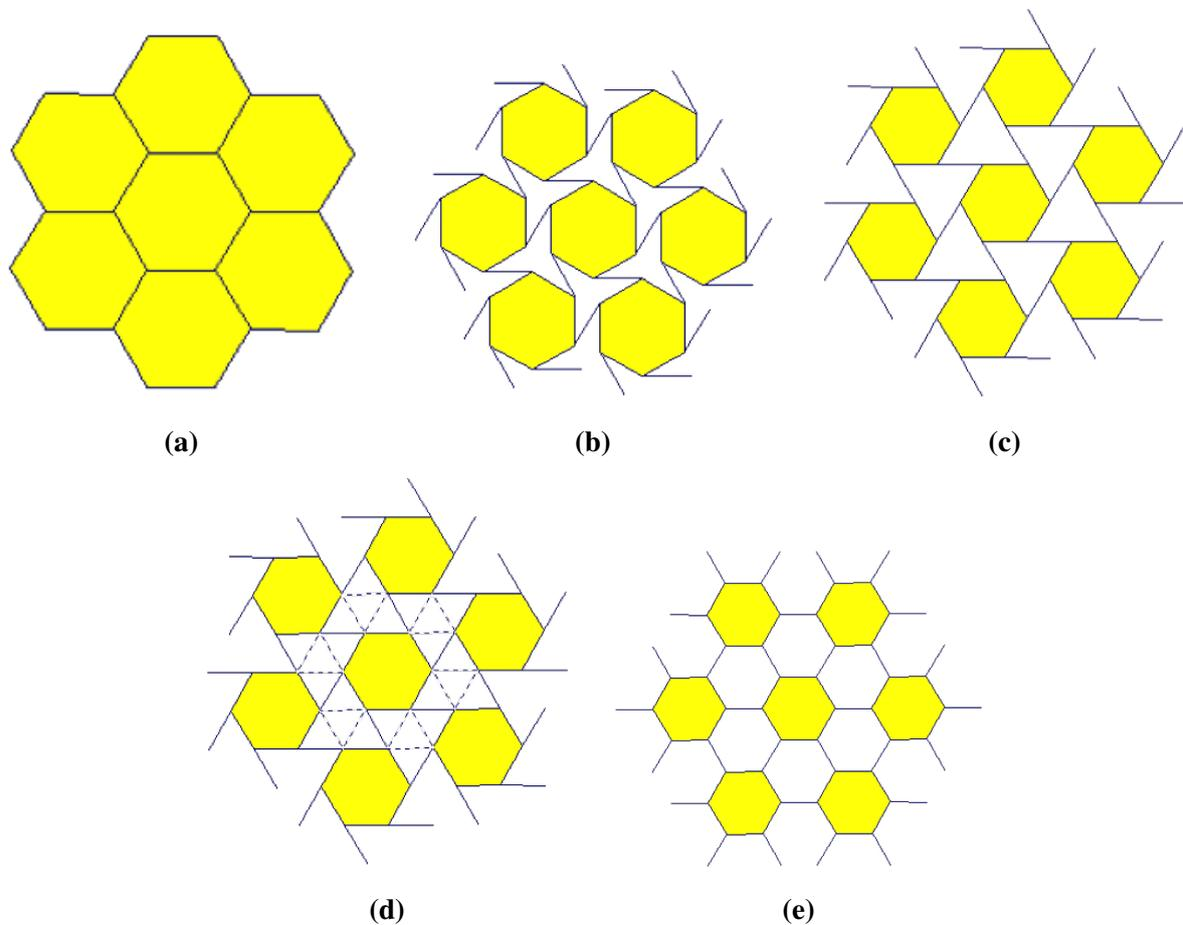
**Figure 8.** Hinged hexagons with rods.
