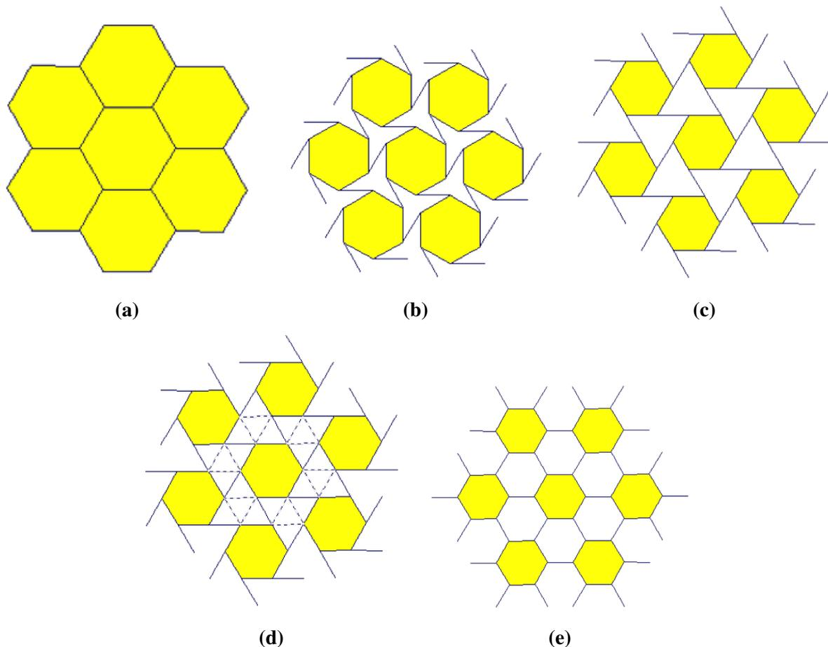
**Figure 8.** Hinged hexagons with rods.
