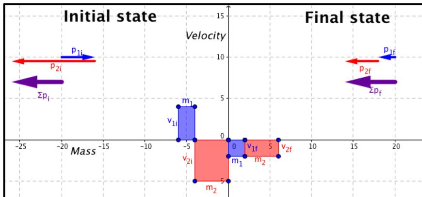
**Figure 2.** Inelastic collision example with initial conditions of  $m_1 = 2$ ,  $\mathbf{v}_{1i} = +4$ ,  $m_2 = 4$ ,  $\mathbf{v}_{2i} = -5$  and solution  $\mathbf{v}_f = -2$ . The final velocity can either be estimated from the grid or numerically from the Algebra panel. With the right units this could represent a head on collision between a sports car going in the opposite direction of a Sport Utility Vehicle (SUV) both traveling at the same speed.
