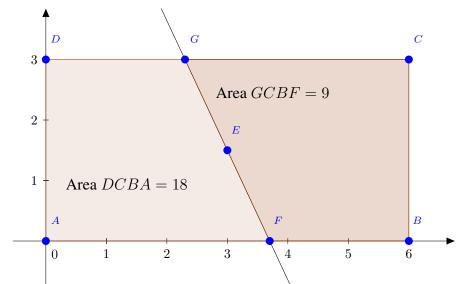
Figure 8. Any line through a rectangle's center divides the rectangle into two equal areas
