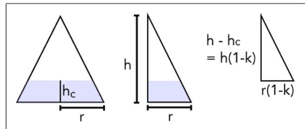
Fig 8: A front view of the liquid in the cone (left), and the two similar triangles (middle and right).
