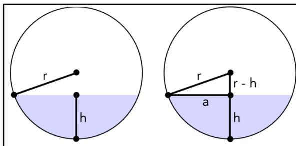
Fig 2: Front views of the liquid in the ball (left), and of the spherical cap (right).
