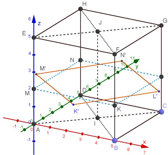
**Figure 2.** Setup for twisting a cube while retaining the volume (the plane containing  $L'K'M'N'$  is not shown; created with GeoGebra®).
