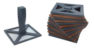
**Figure 10.** A cube is sliced for modeling the twisting process; the twisted center prism provides rotational guidance (created with Autodesk Fusion  $360^{\text{(B)}}$ ).
